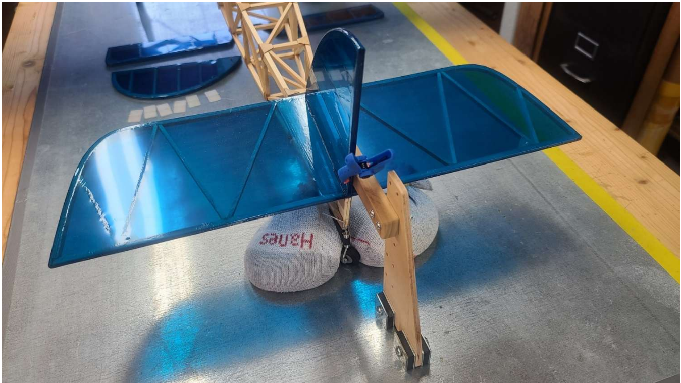
Figure 35 - Vertical Stabilizer Installation
