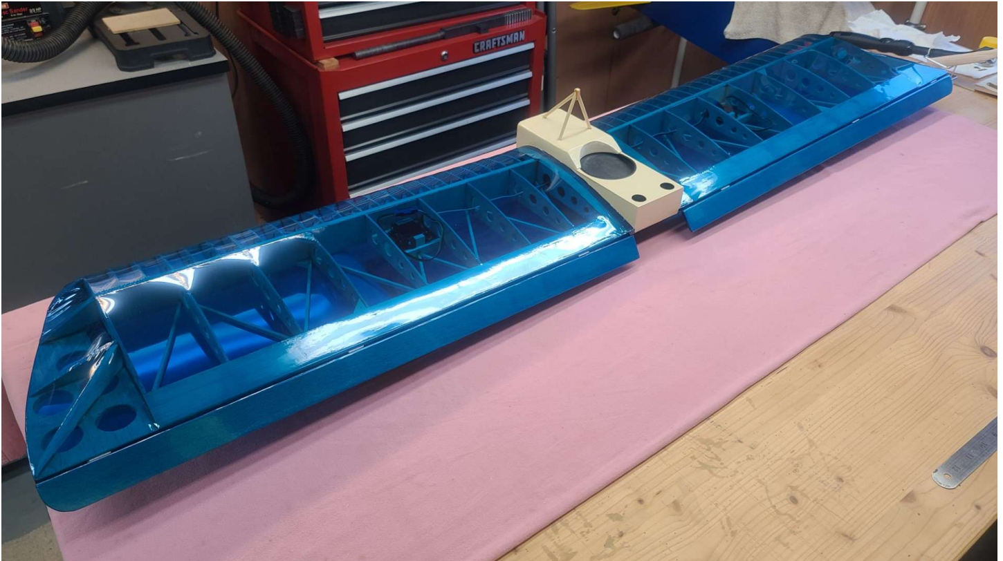
Figure 31 - Miss Vintage Wing Covering Completed
