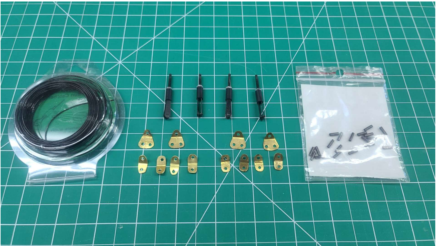
Figure 32 - Wing Rigging Wires Hardware
