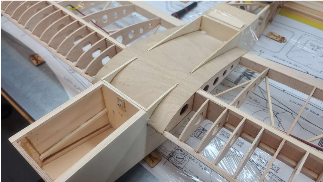
Figure 16 - Wing Bolt-On Installation
