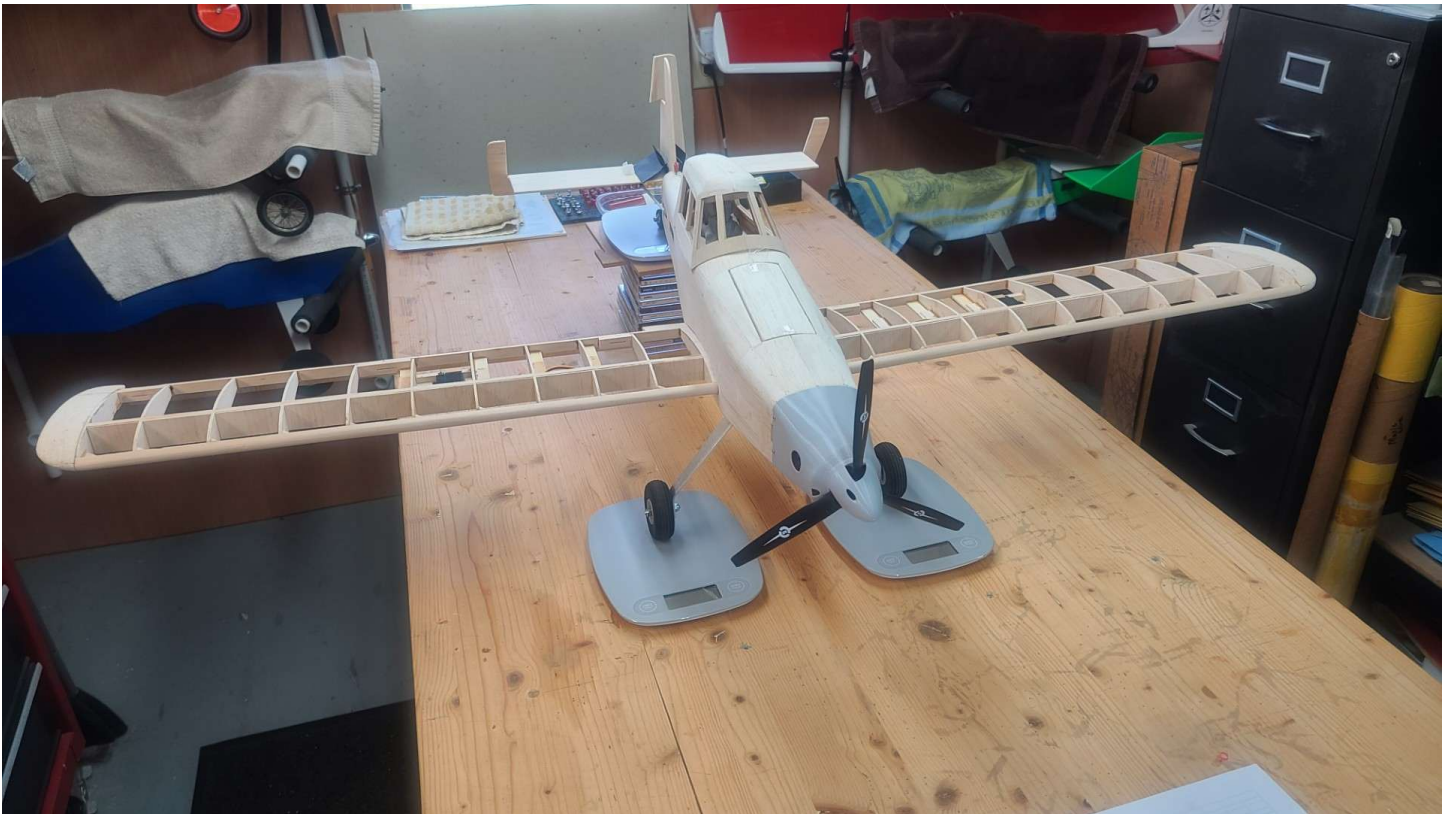
Figure 59 - Full-up Fit Check & CG Measurement
