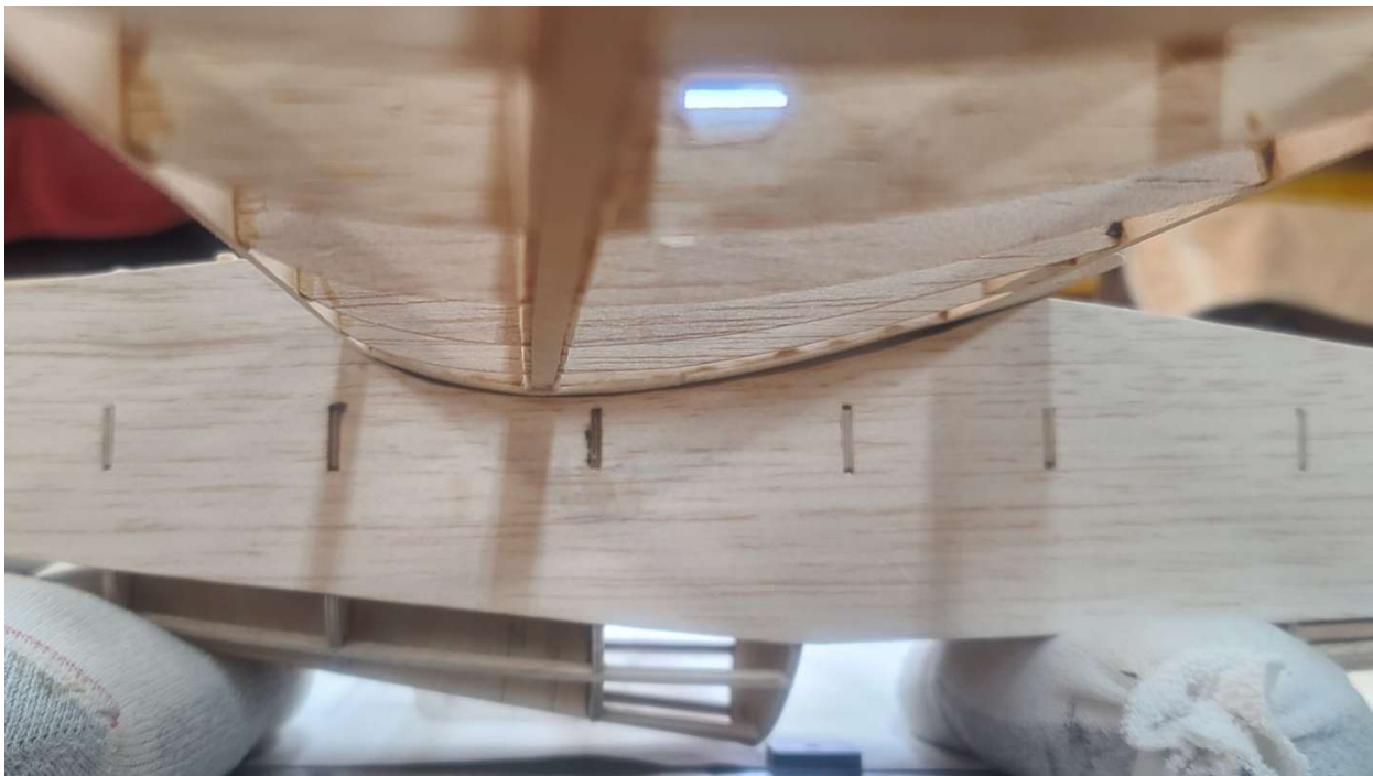
Figure 37 - OA-1K Wing to Fuselage Wing Saddle Fit
