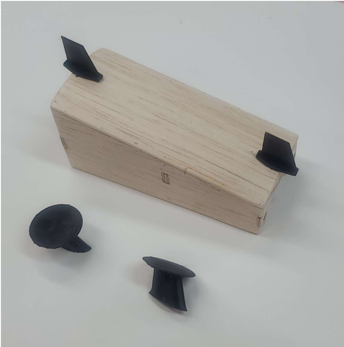
Figures 58 - OA-1K 3D Printed Communications Antennas
