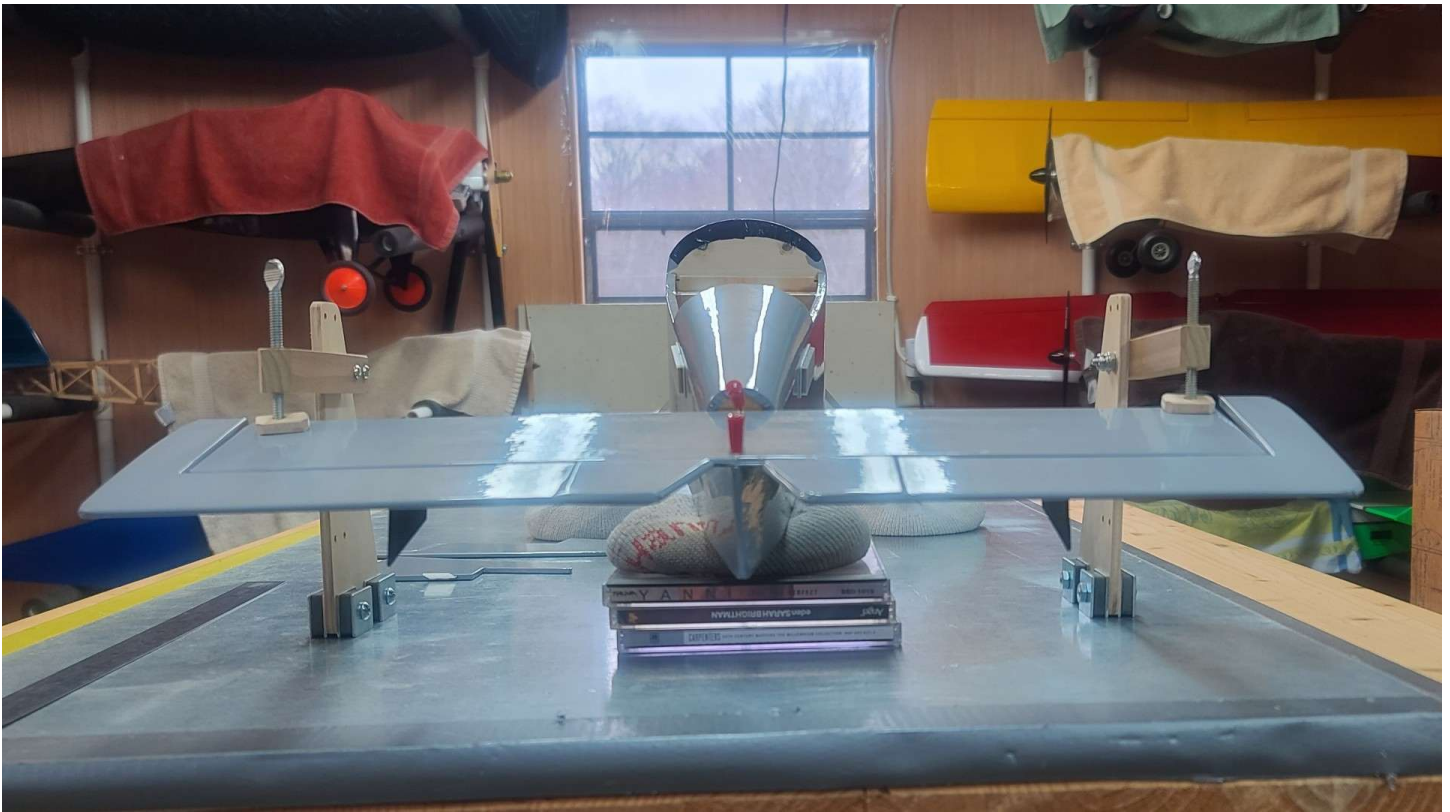
Figure 70 - Horizontal Stabilizer to Fuselage Join
