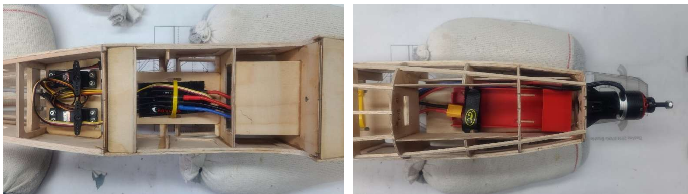
Figure 41 - ESC to Motor Cable Routing
