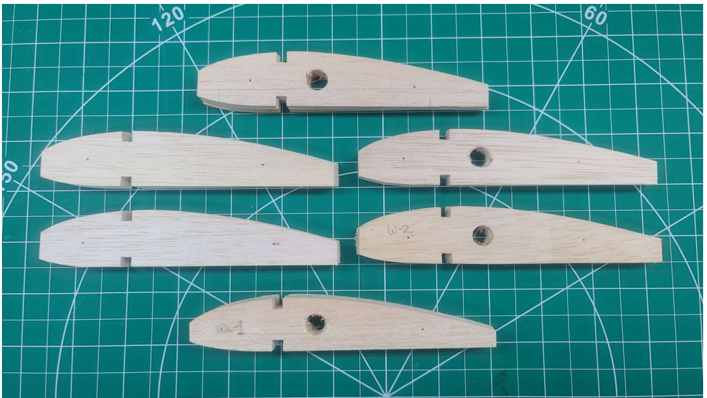
Figure 16 - OA-1K NACA 4415 Airfoil Profile Wing Ribs (24 total)
