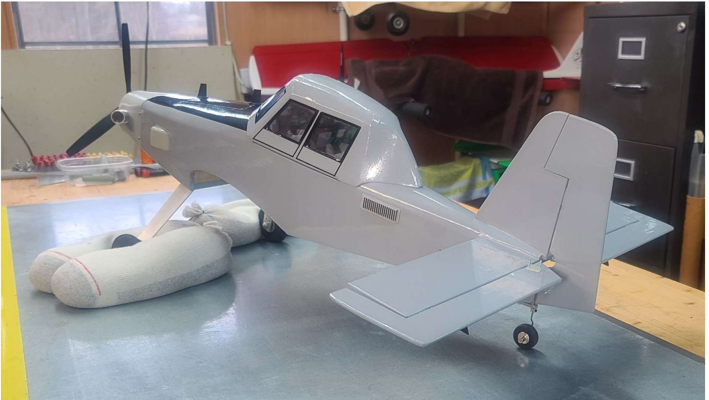
Figure 71 - Vertical Stabilizer & Tail Wheel Installation
