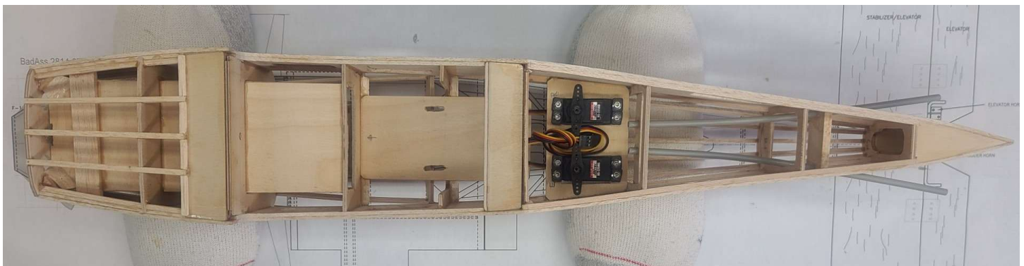
Figure 35 - OA-1K Fuselage Assembly Bottom View (cont.)
