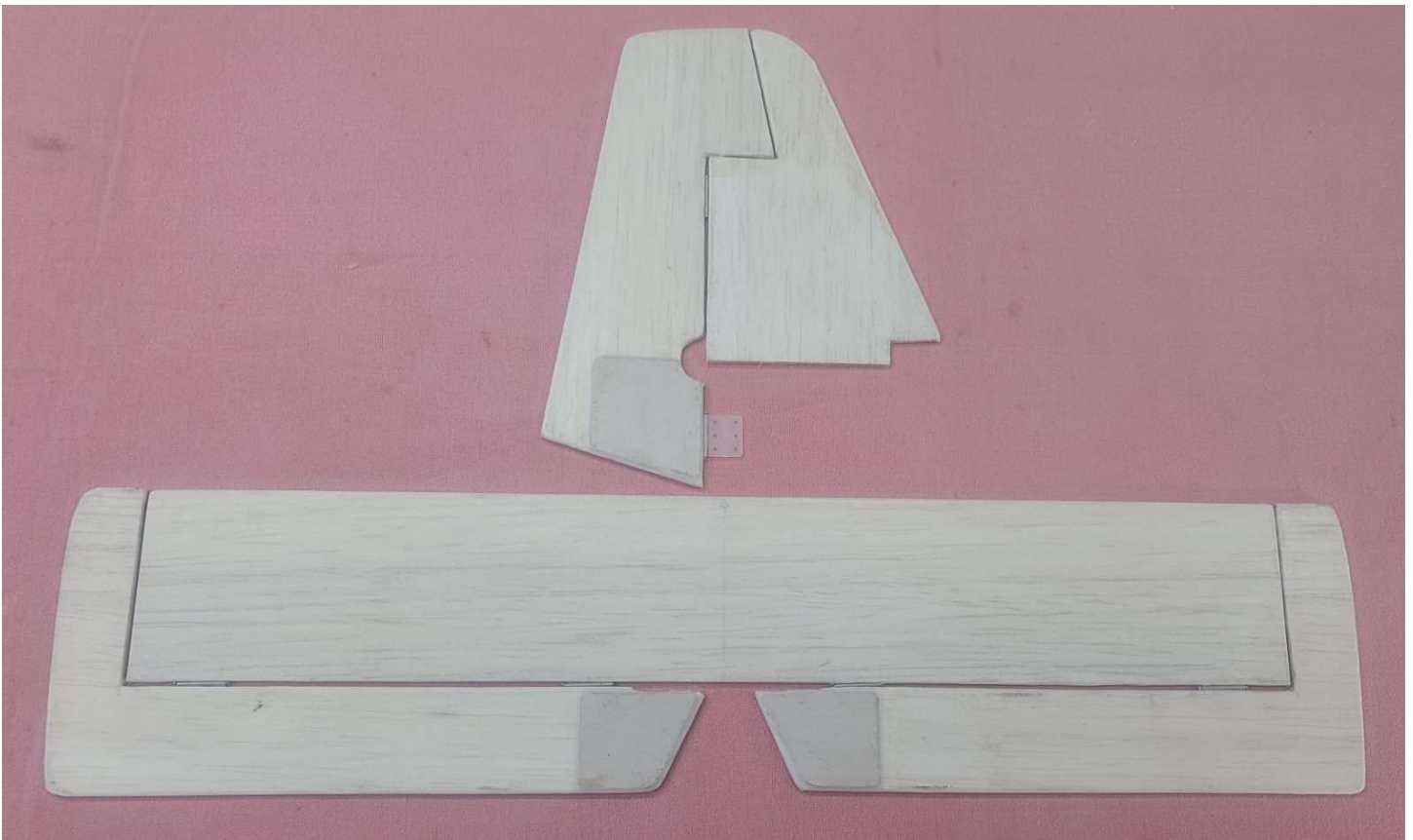
Figure 63 - OA-1K Tail Feathers Covered with SIG Koverall
