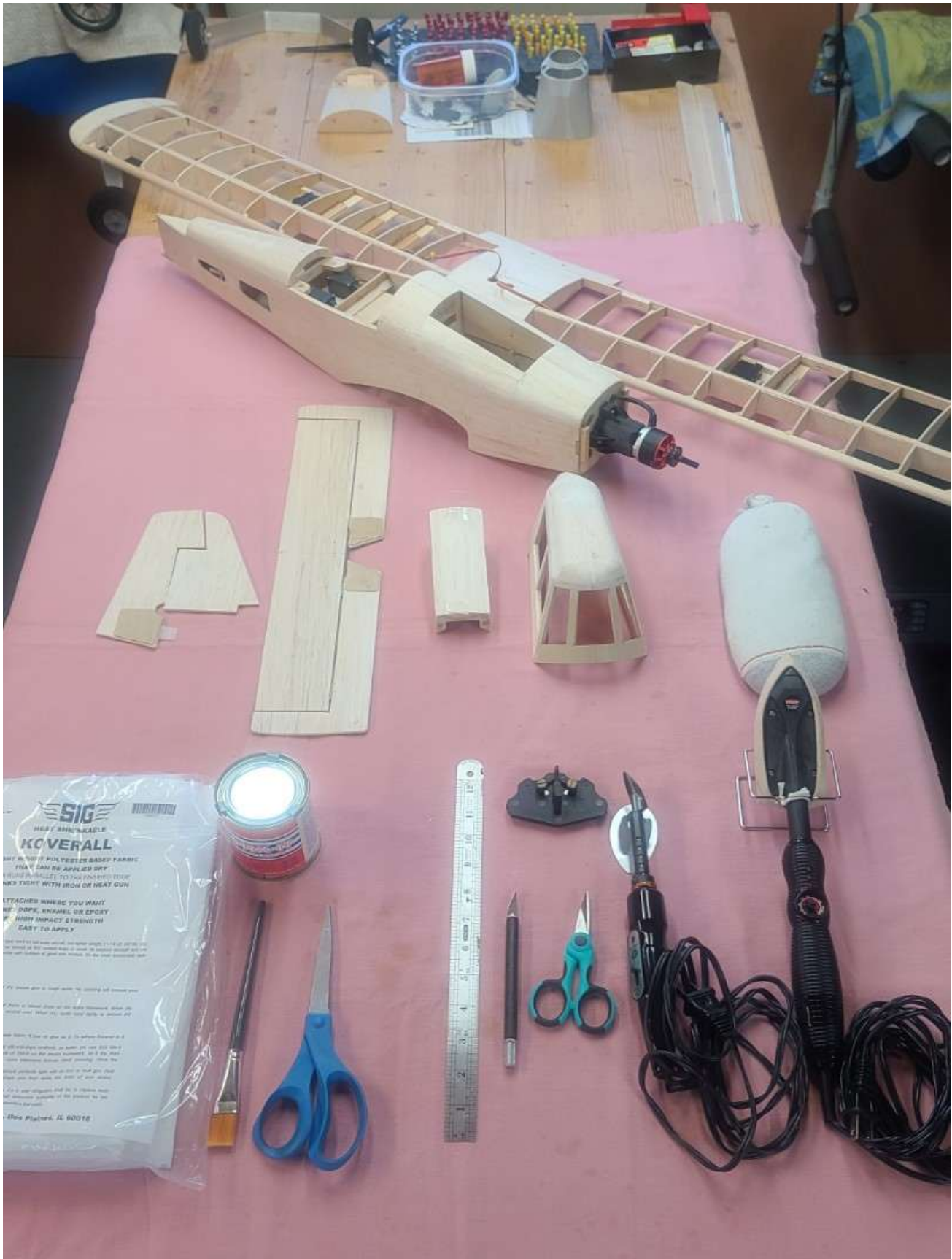
Figure 62 - OA-1K Covering Set-Up, Required Tools & Materials
