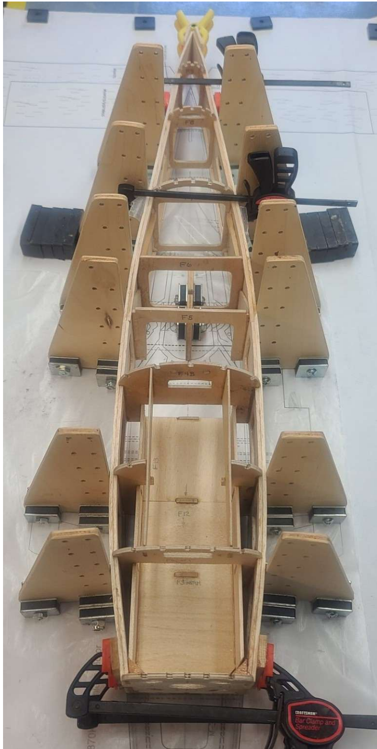
Figure 34 - OA-1K Fuselage F2, F7-F9 Assembly
