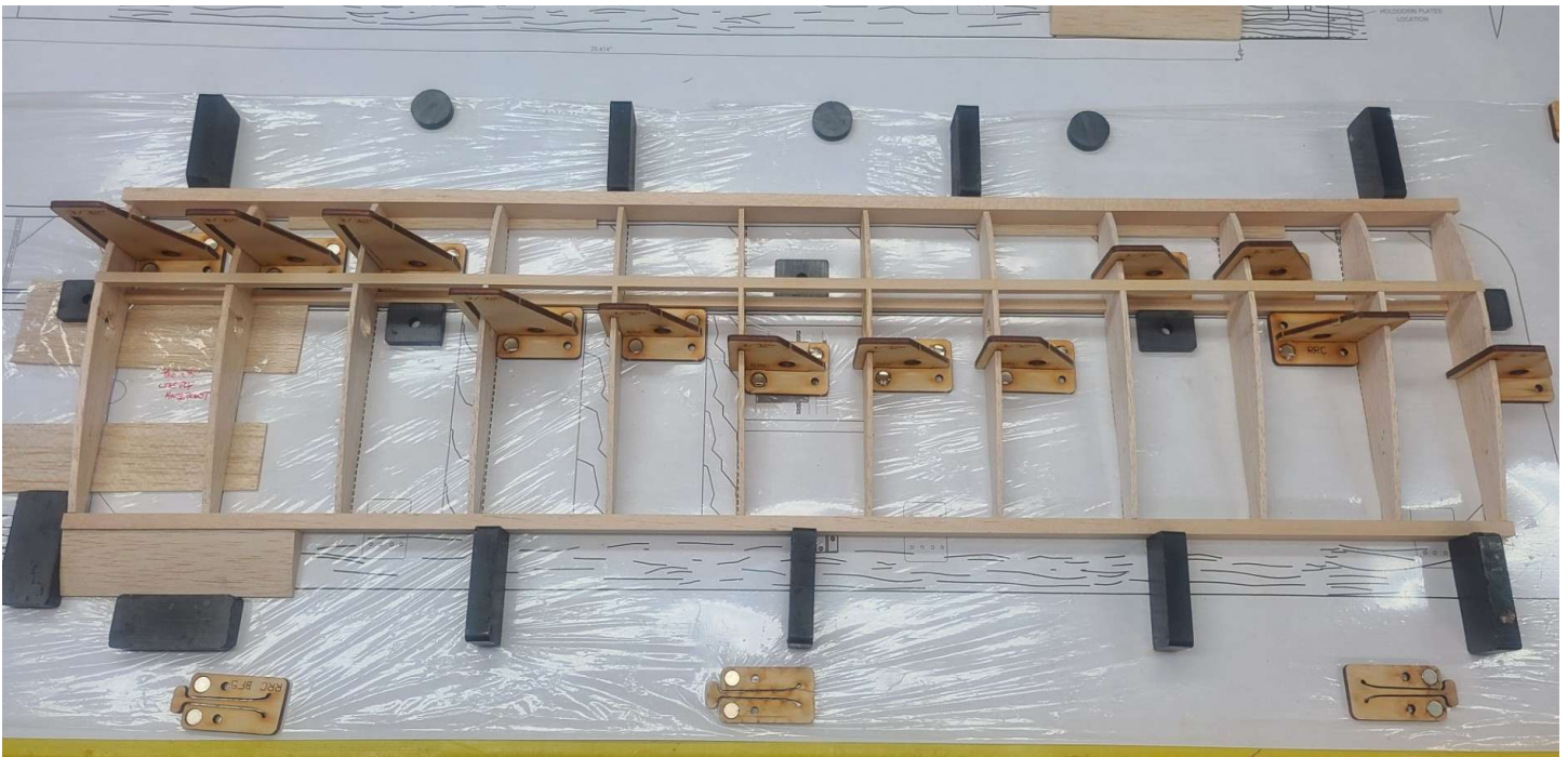
Figure 17 - OA-1K Wing Right Half Full-Up Dry Run Fit Check on Magnetic Build Board
