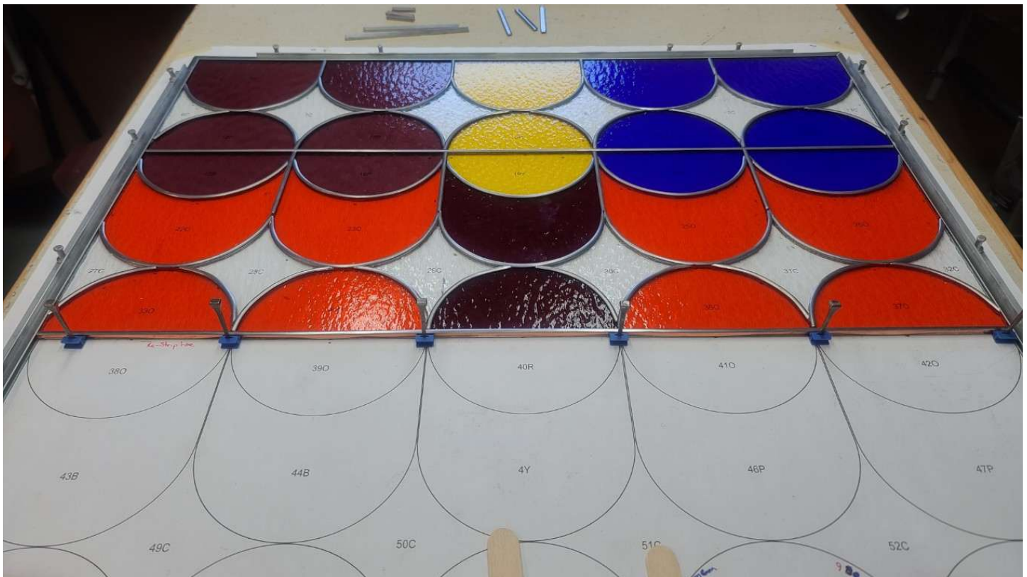
Figure 11 - Continuing the Panel Assembly
