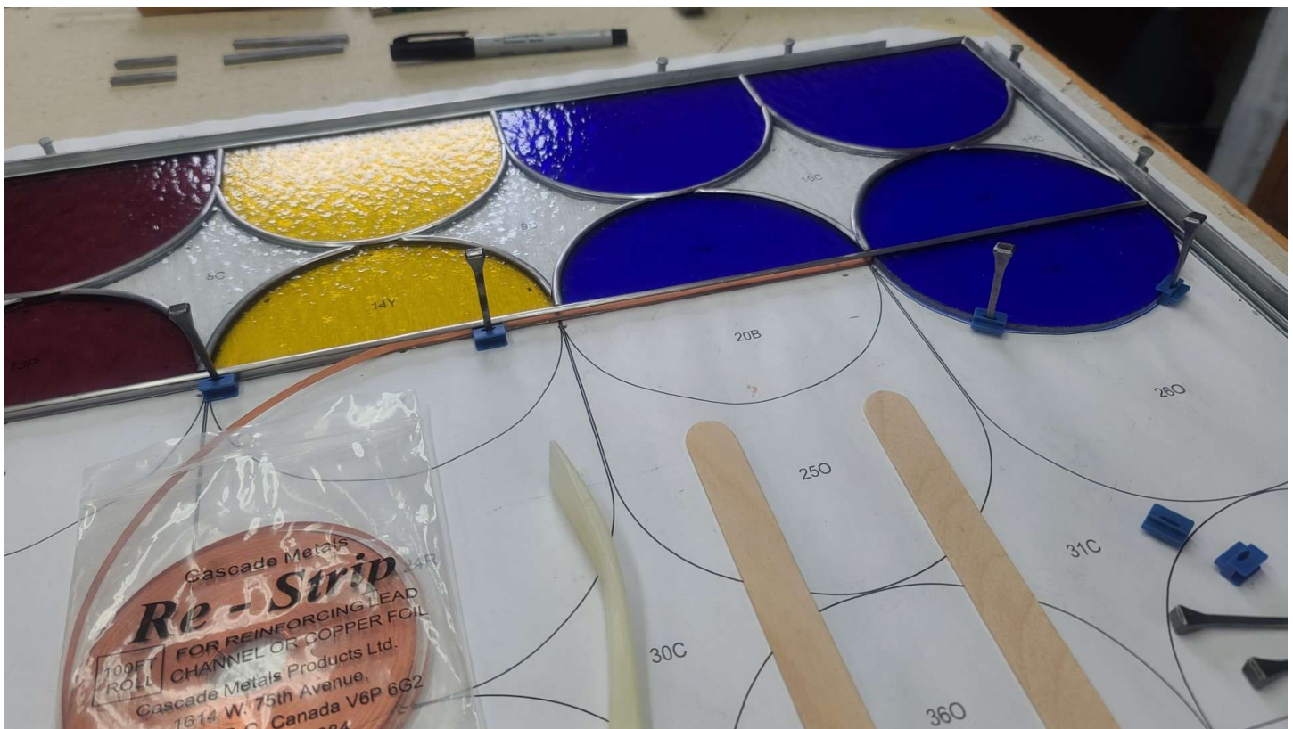
Figure 10 - Re-Strip Inside the Lead H-came
