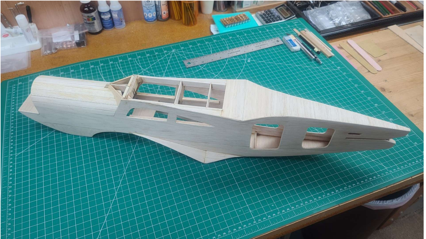
Figure 54 - Stagger Bee II Fuselage Ready for Ultracoat Covering
