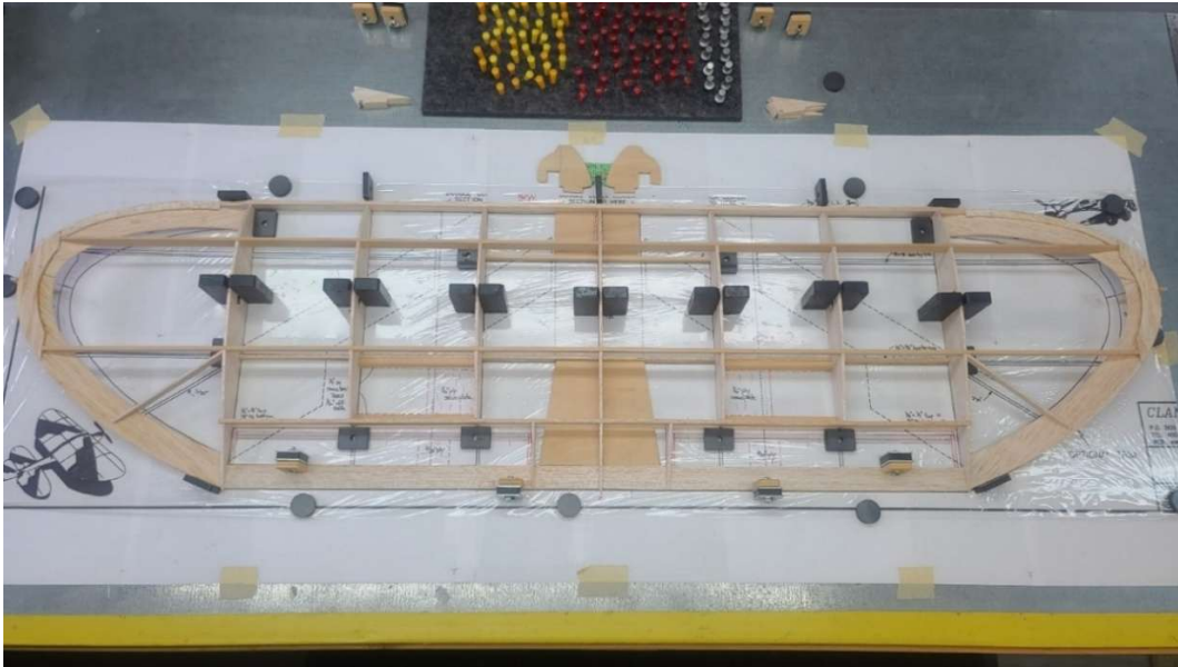
Figure 8 - Modified Top Wing Full-Up Dry Fit Check on Magnetic Build Board
