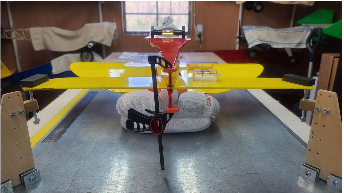
Figure 43 - Horizontal Stabilizer Installation
