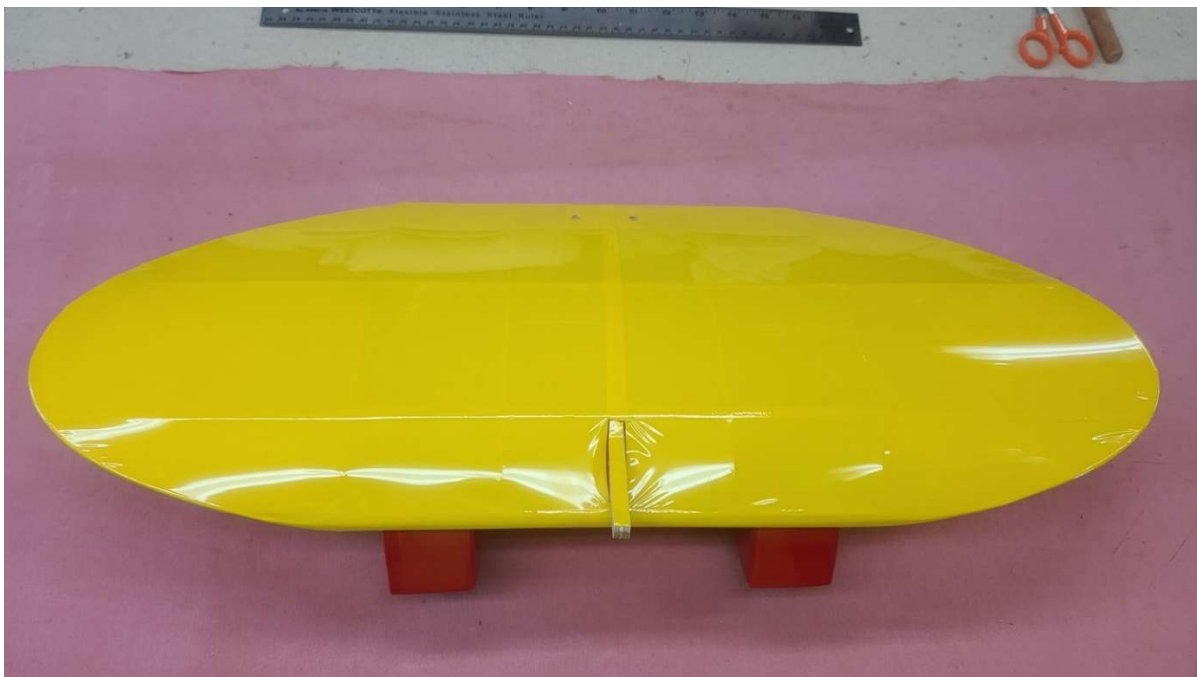
Figure 38 - Bottom Wing Covering Completed
