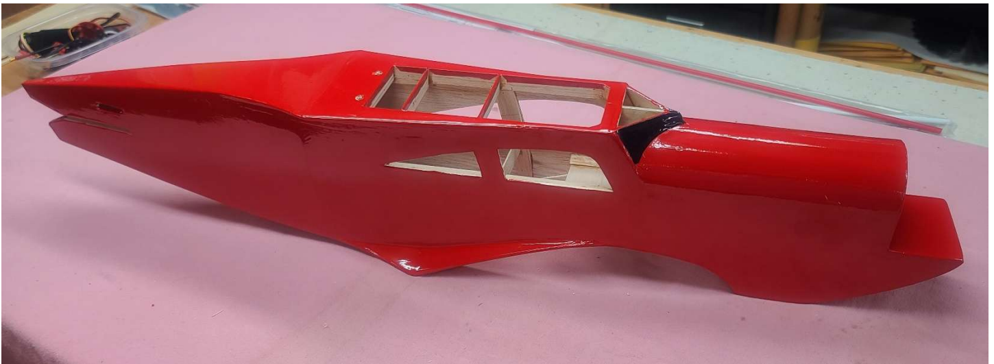
Figure 55 - Stagger Bee II Fuselage Covering Completed
