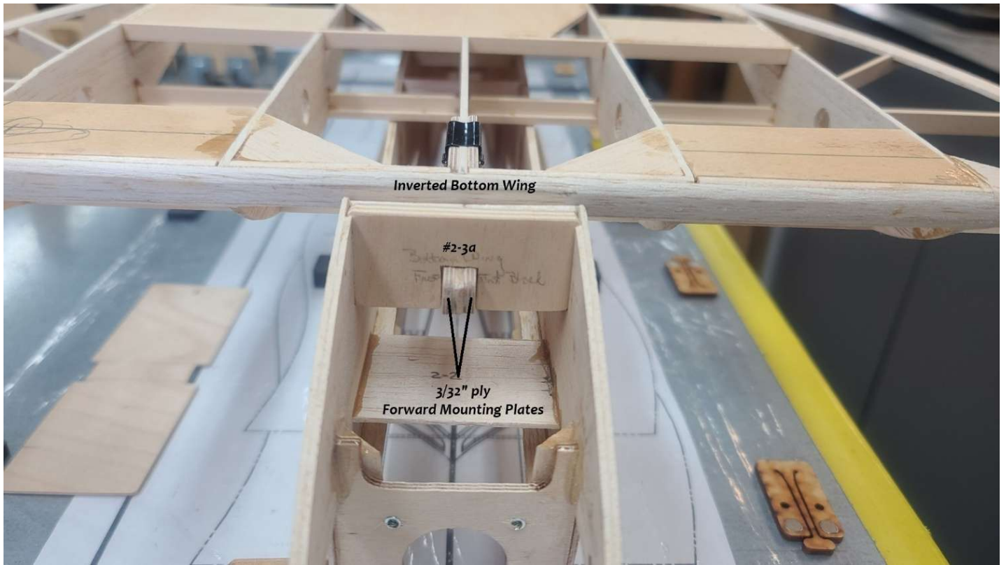
Figure 21 - Bottom Wing Forward Mounting Plates to Fuselage Part #2-3a Fitting
