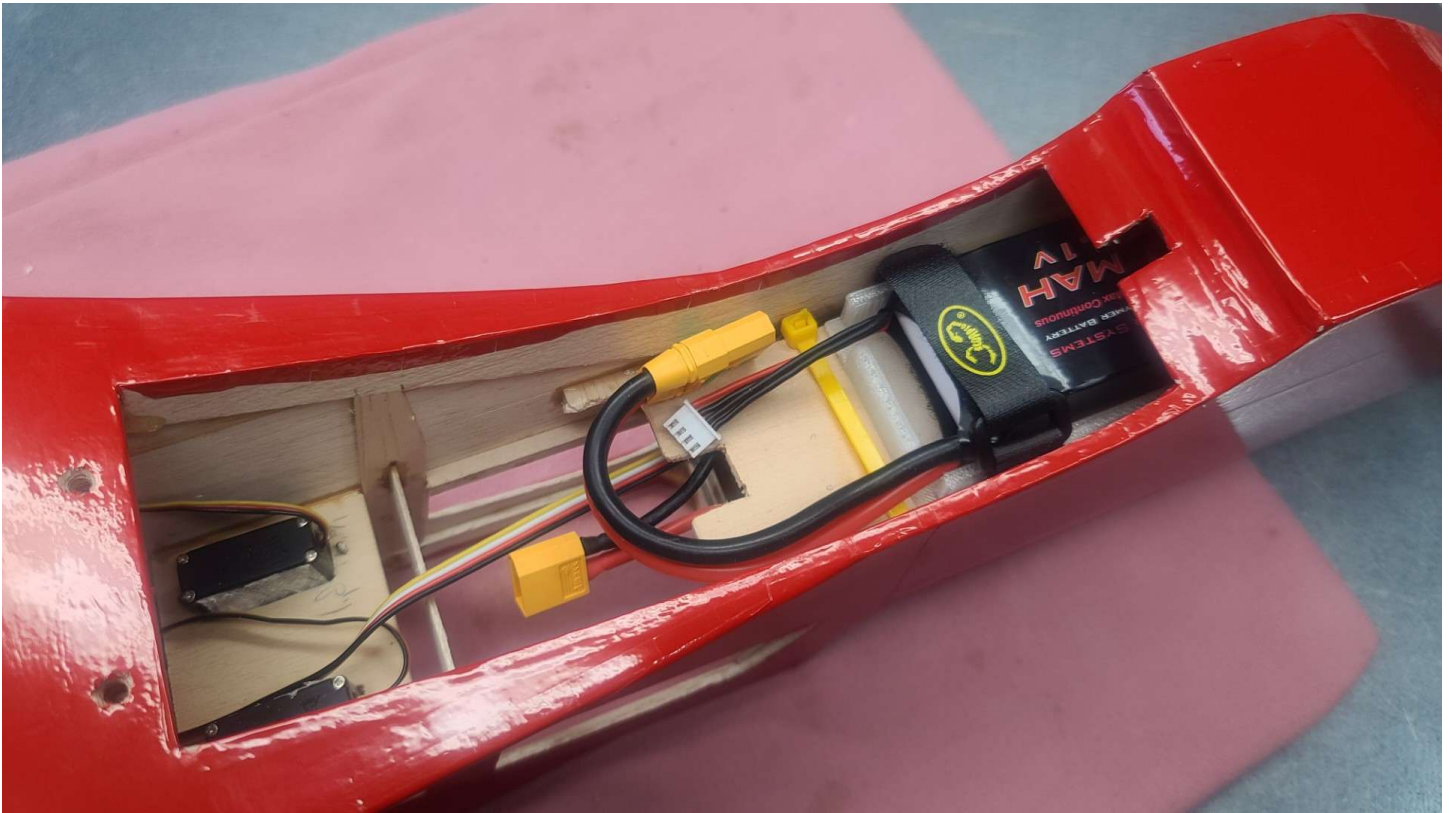
Figures 56 & 57 - 3D Printed LiPo Battery Mounting Tray
