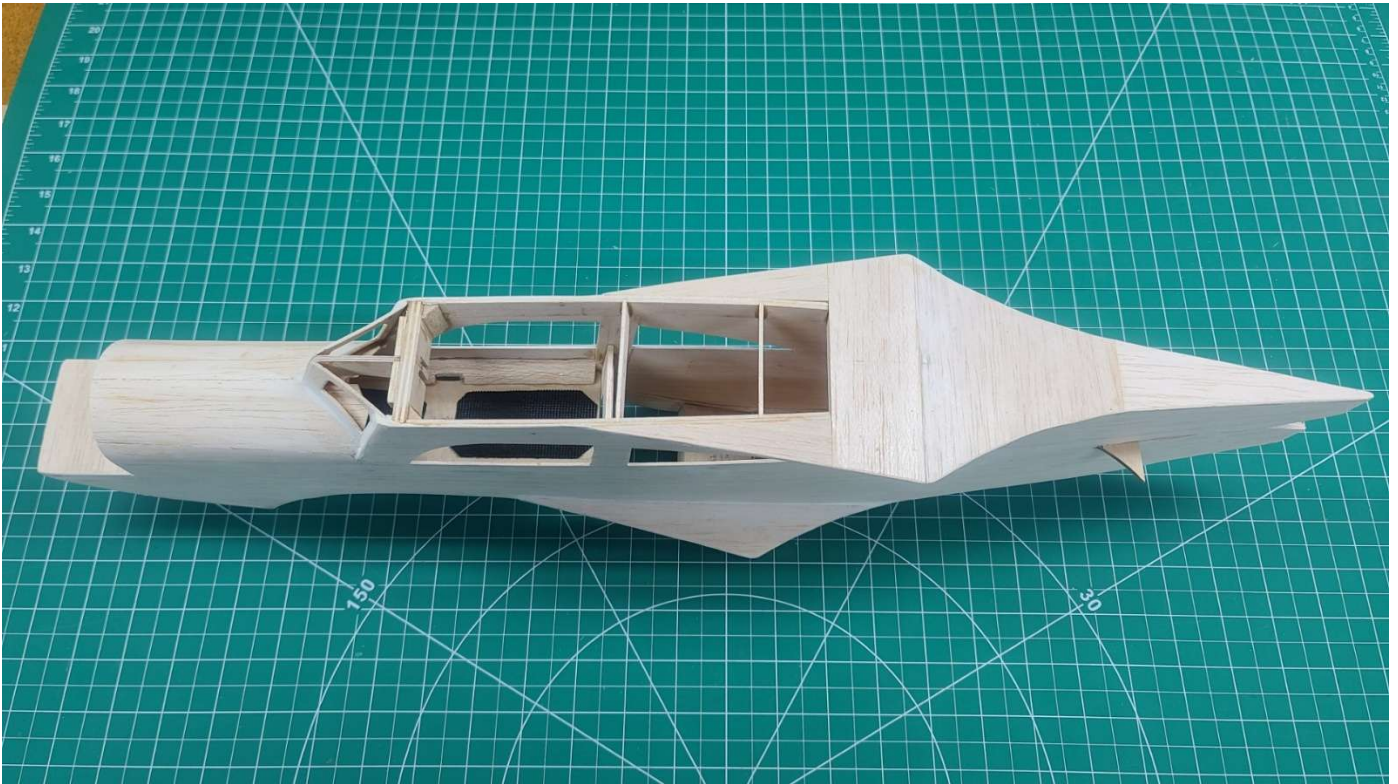
Figure 24 - Fuselage Top Sheeting
