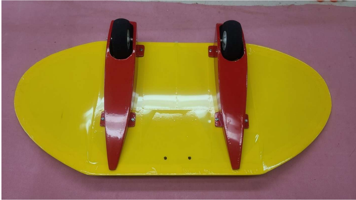
Figure 39 - MLG Wheel Skirts Installation
