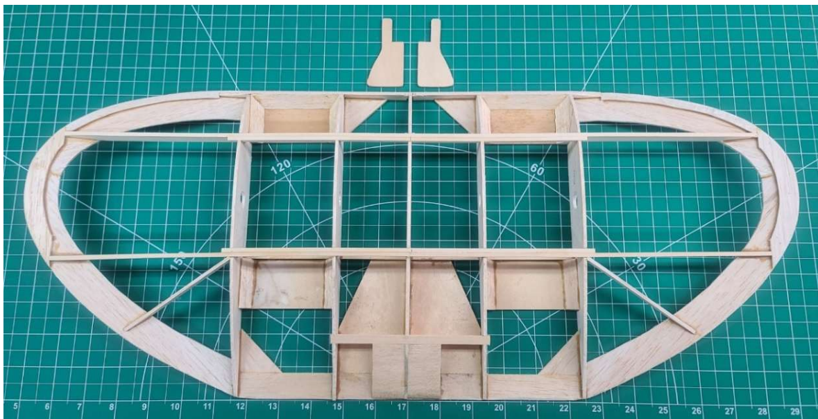
Figure 14 - Modified Bottom Wing
