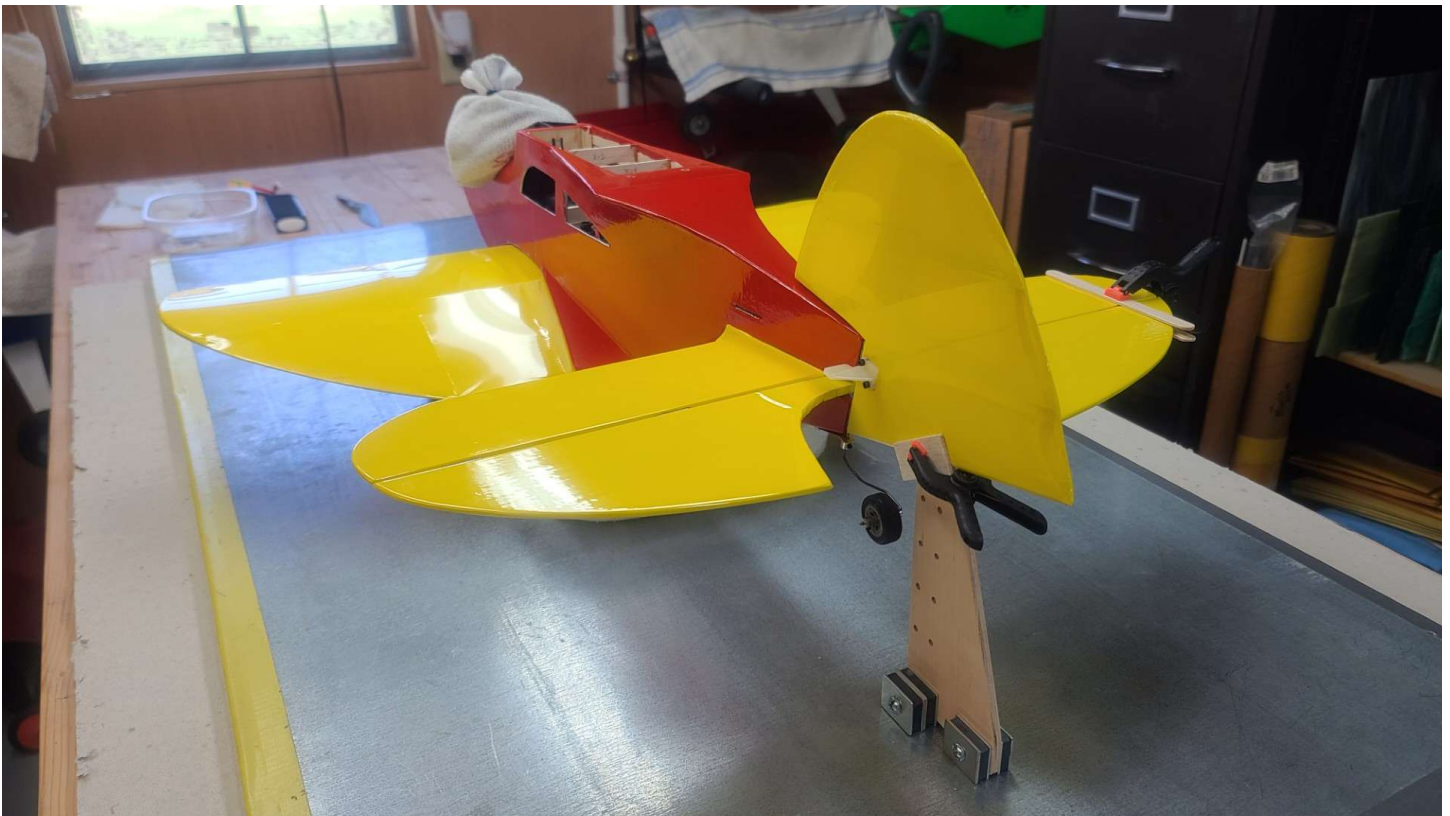
Figure 44 - Vertical Stabilizer/Rudder Installation
