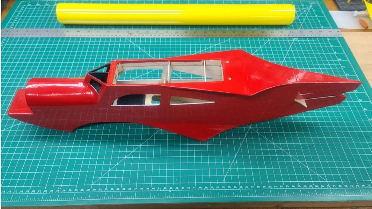
Figure 37 - Fuselage Covering Completed
