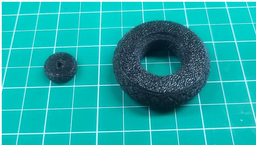
Figure 13 - Belly Wheel and Tailwheel Tire Parts using TPU
