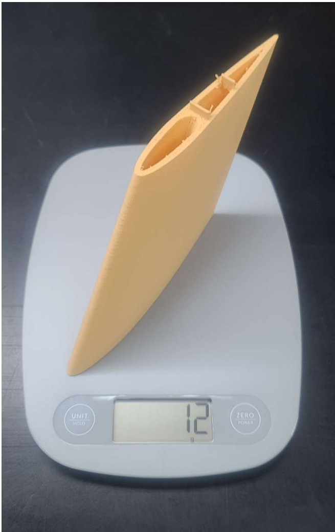
Figure 8 - Vertical Stabilizer & Fuselage 4 3D Print Using Polylight 1.0 LW-PLA (Balsa)
