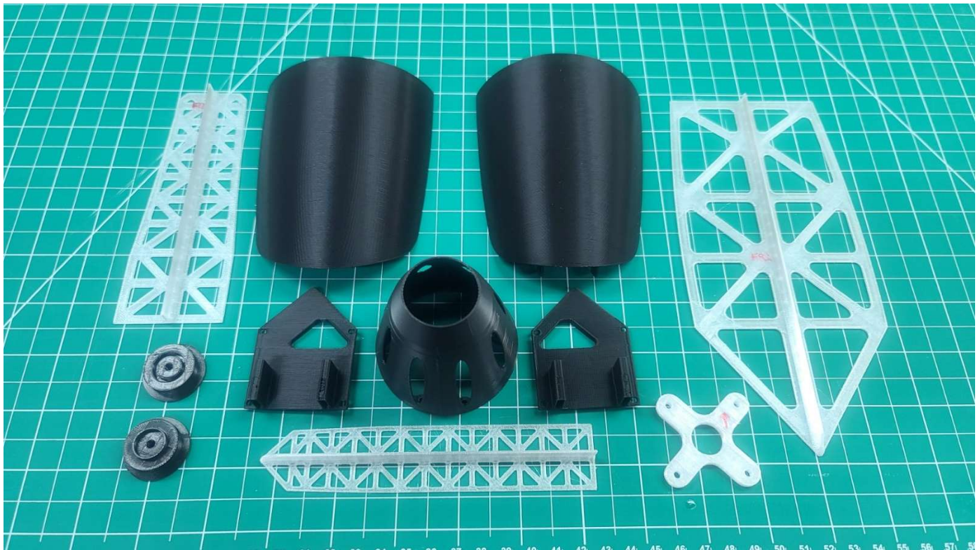
Figure 4 - X-100 Infinity Wing V2 3D Printed PLA & PETG Parts
