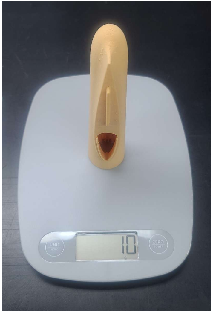
Figure 8 - Vertical Stabilizer & Fuselage 4 3D Print Using Polylight 1.0 LW-PLA (Balsa)
