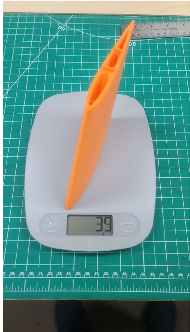
Figure 6 - Vertical Stabilizer 3D Prints Using Hyper-PLA (white) & Air PLA (orange)
